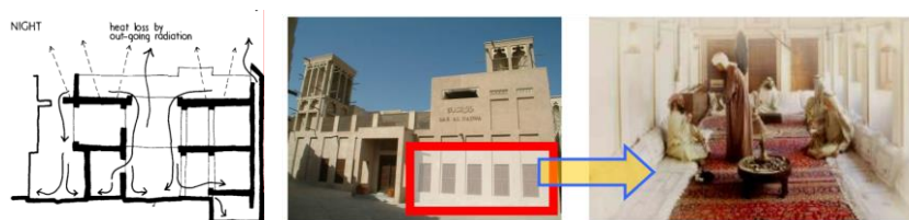
Figure 95 (i) Thermal performance of the courtyard in a traditional house (ii) Extrovert looking openings
