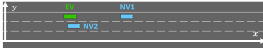
Figure 26: Textual requirement of slower action ( TRQ2 ): The EV shall decelerate smoothly when it is in the the 3rd lane (left lane) and surrounded by at least two cars: the first at least 20 meters in front, the second at least 7 meters to the right, provided that the relative speed of all surrounding vehicles is within the range of -2.5 m/s to 1.5 m/s for a continuous period of at least 5 timesteps.
