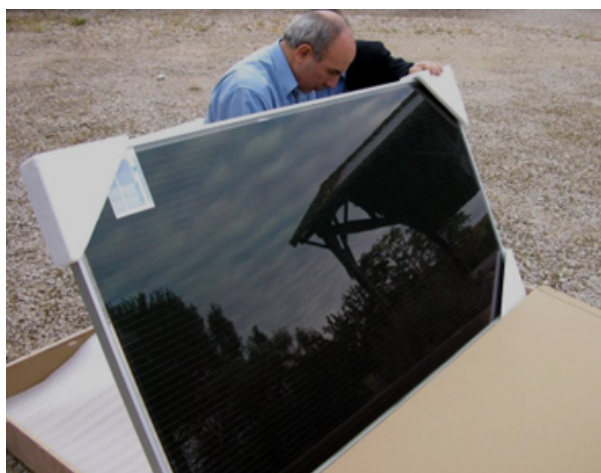
FIGURE I.5 – Cellule au Silicium amorphe (couche mince) [9]
