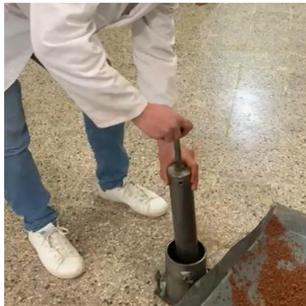
Figure 3.1 : Essai de compactage Proctor
