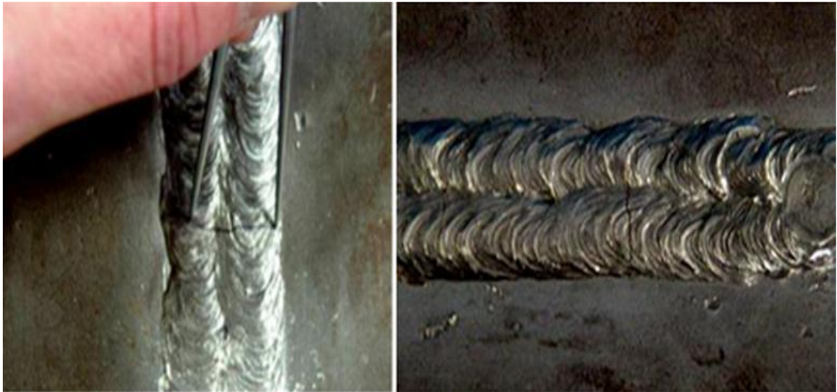
Figure 18 : La fissure transversale. [11]
