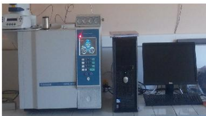
Figure II.7: Appareil CPG " YL instrument 6500 GC system".
