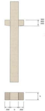
Figure 75 : poteau a consoles
