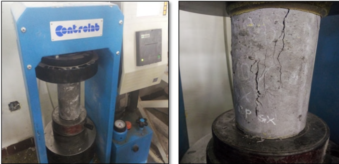
Figure IV.18. Essai de compression.
