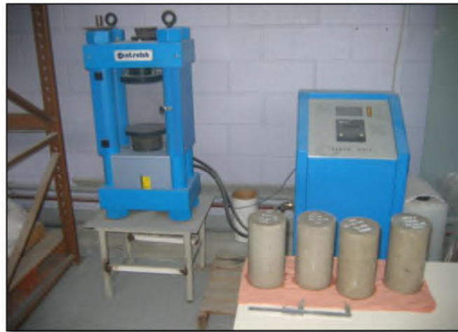
Figure I.2. Essai de compression (Khelifa, 2009).
