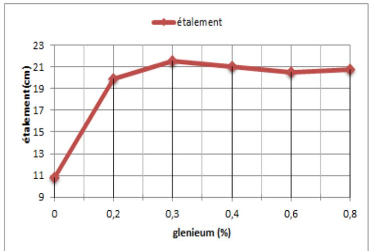
Figure 3.11: courbe dosage de saturation (mini cône)
