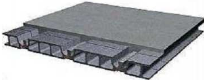
Figure 1.3 Plancher corps creux
