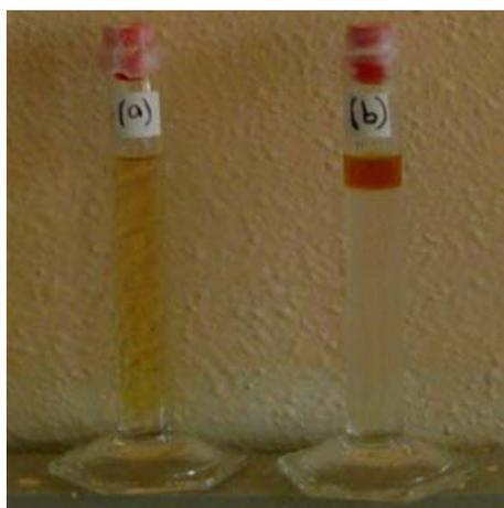
**Figure 1.** Cloud Point Extraction of uranyl ions in acetate medium, in presence of (I)
