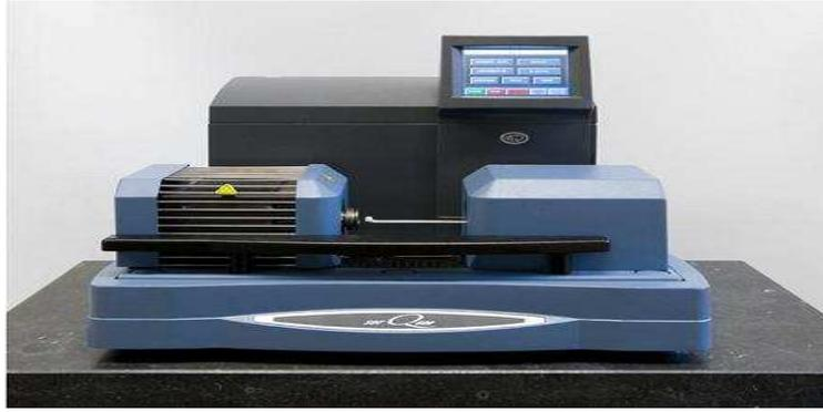
**Figure 1** : Appareil TA Instrument SDT Q600
