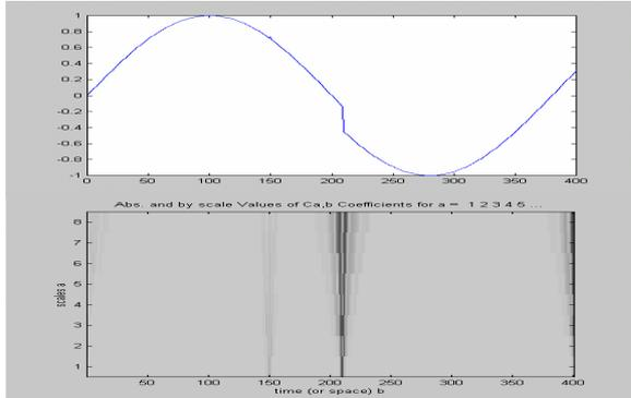
Figure 2 : Application of the CFT (middle) and CWT (bottom) to transient signal (top)
