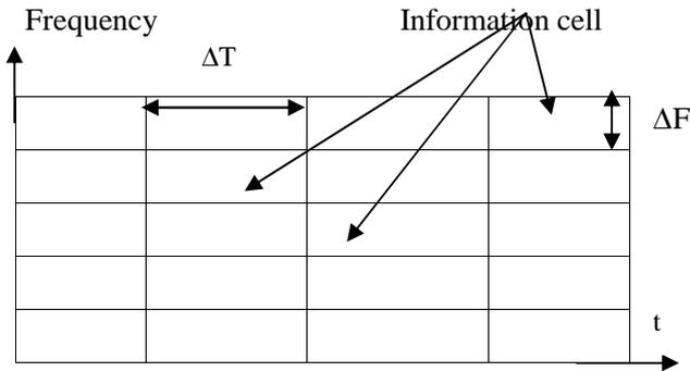
Figure 1 : time-frequency view of the signal -STFT-.
