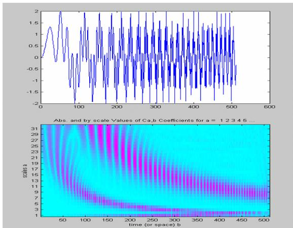
Figure 3 : Application of the CFT (middle) and the CWT (middle) to the chirp signal (top)
