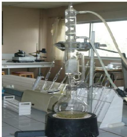
**Figure 10 :Appareil Soxhlet**
