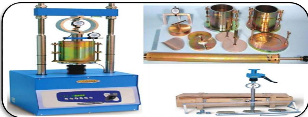
**Figure 3.4 :** Essai C.B.R.
