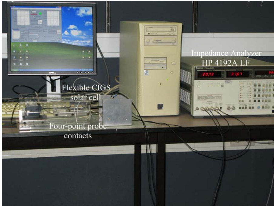
Figure 11 Setup of C - V and C - f measurement used at ELIS.
