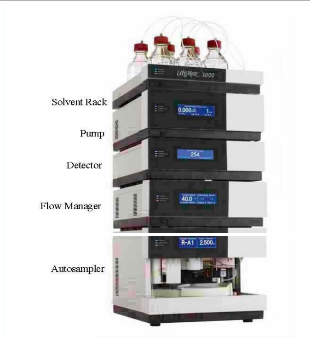
Figure 2. 8 : Ultimate 3000 de LC-Packing Dionex
