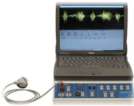
Figure.1.7: Phonocardiographe Cardiosim IV (Cardionics, Inc.) [8]
