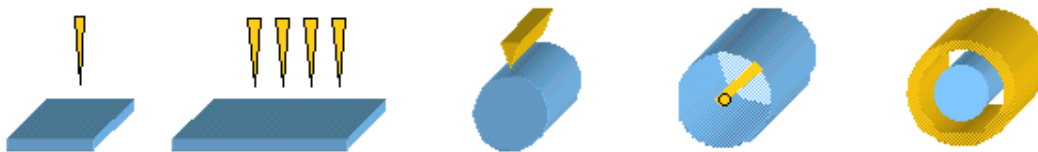
Pointe/Plan Multipointe/Plan Couteau/Cylindre Fil/Cylindre Cylindre/Cylindre
