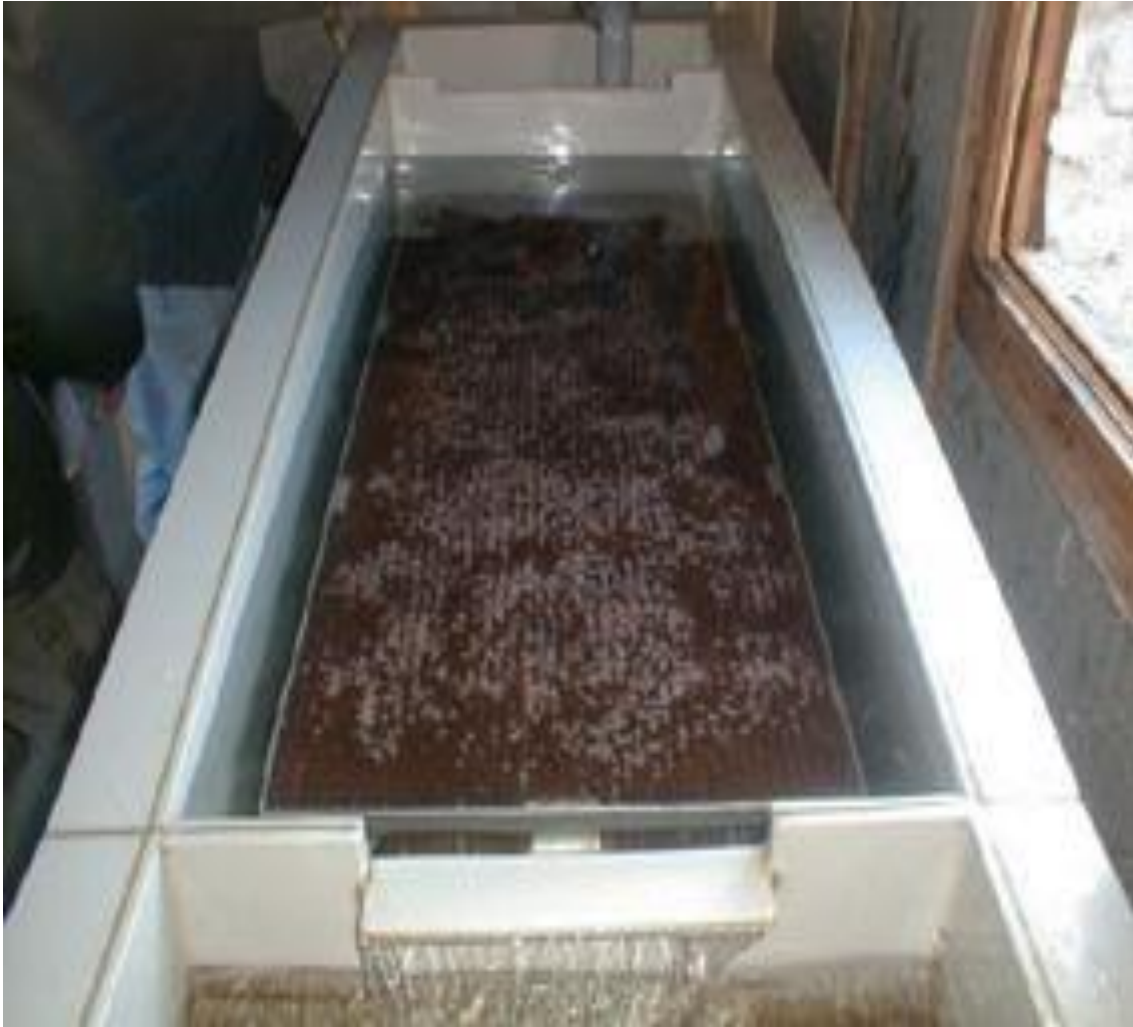
An incubator that can accommodate 50,000 salmon eggs
