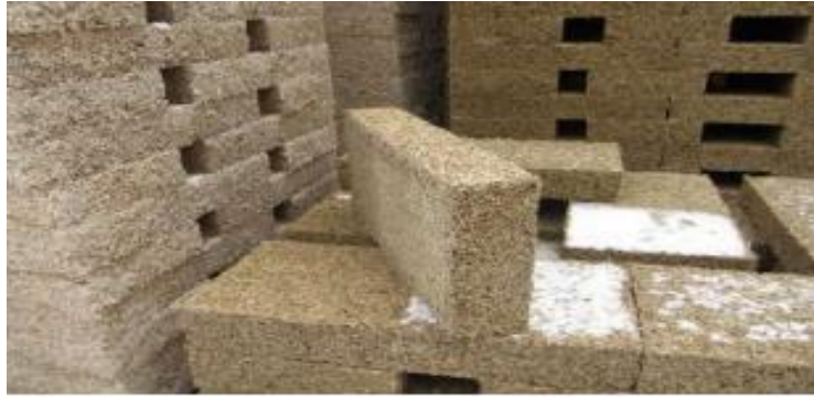
Figure 12: Béton de chanvre [20]
