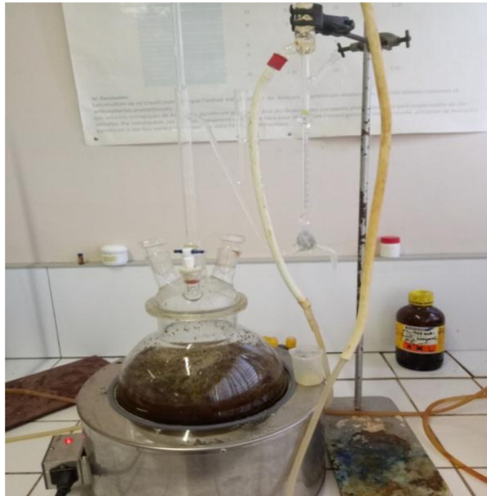
Figure 6: Montage de l'hydrodistillation type Clevenger
