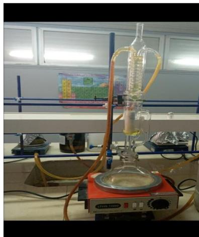
*Figure 11: montage de soxhlet*
