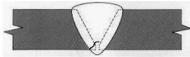
Figure III.10: Fissure de Racine
