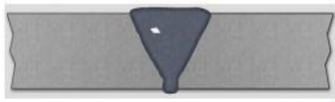
Figure III.32 : Inclusions de cuivre
