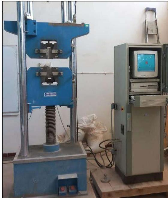
**Figure III.5:** Machine de traction.
