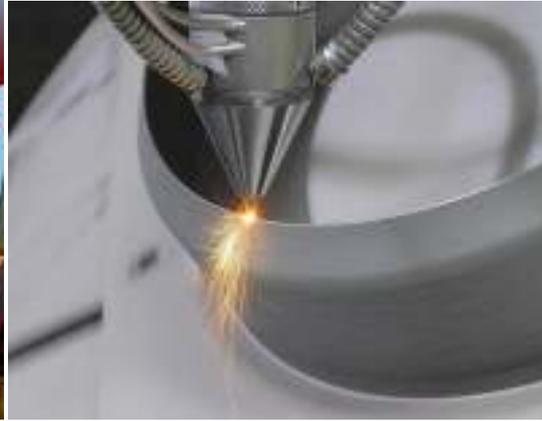
Figure 1.19: Fabrication additive Impression 3D
