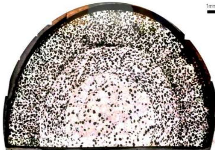
Figure I-3: A top view of a radial cross-section of a cylinder showing graded porosity distribution in the radial direction [27]
