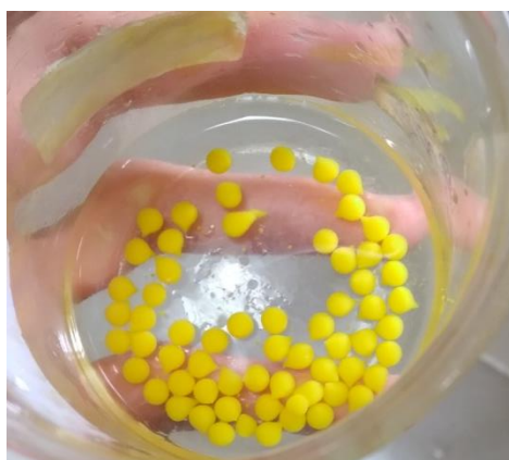
Figure 65 CaCl 2 2% (w/v) cross-linking solution containing the free drug remained and curcuminoids beads
