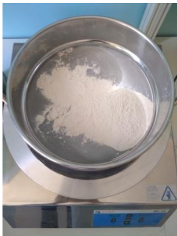
Figure 33 Sieving of Raw Bentonite
