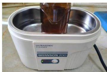
Figure 30 Ultrasound assisted extraction of curcuminoids by acetone
