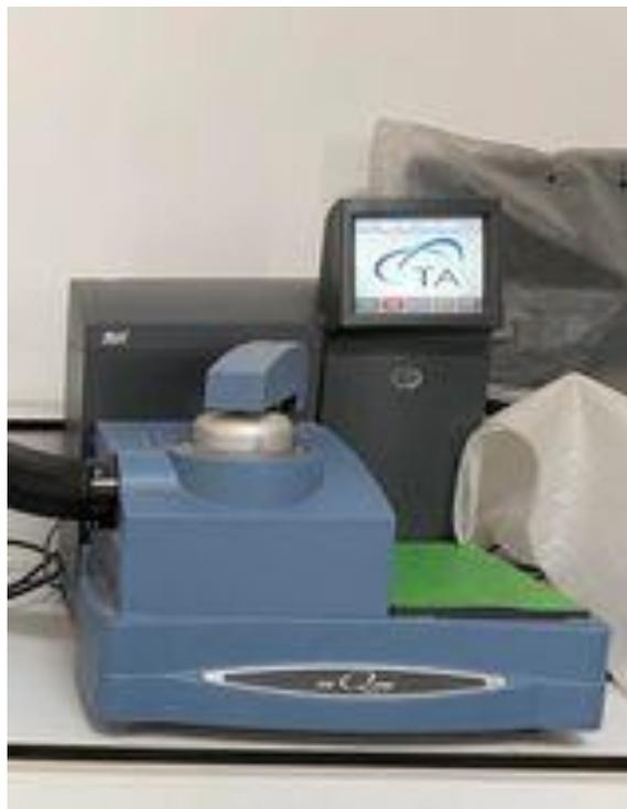
**Figure II.6 :** Appareillage DSC.
