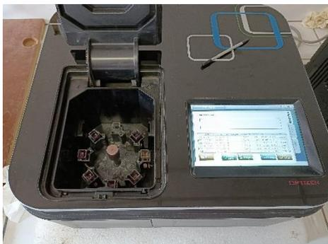
**Figure III- 11:** Appareil UV-Visible
