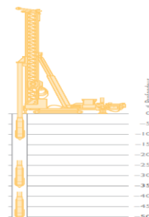
Figure 1.13:vibro-compactage a 50m (keller)
