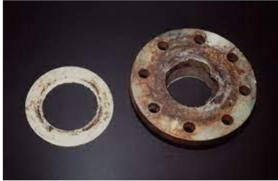
Figure 1. 5: La corrosion caverneuse [9]
