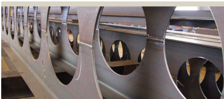
Figure SEQ Figure \* ARABIC 90:poutre alvéolé
