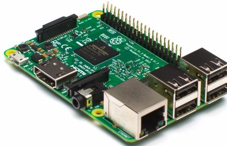
FIGURE IV.2 – Raspberry Pi 3 Model B
