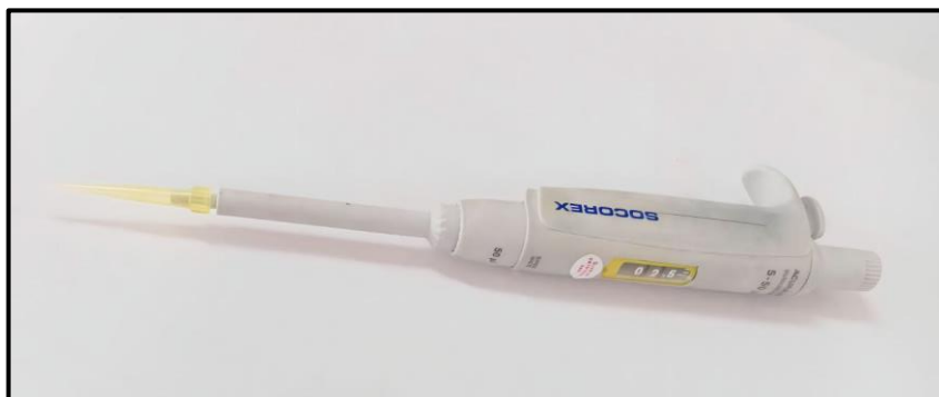
Figure 23 : Micro pipette 5-50ul (photo originale)
