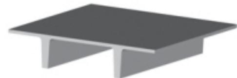
Figure 121 Plancher double nervurer
