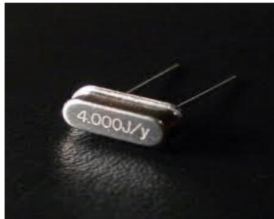
**Figure II.4 Boîtier Quartz [5]**
