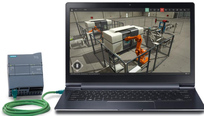
FIGURE 3.24 – Factory I/O et L'API S7-1200
