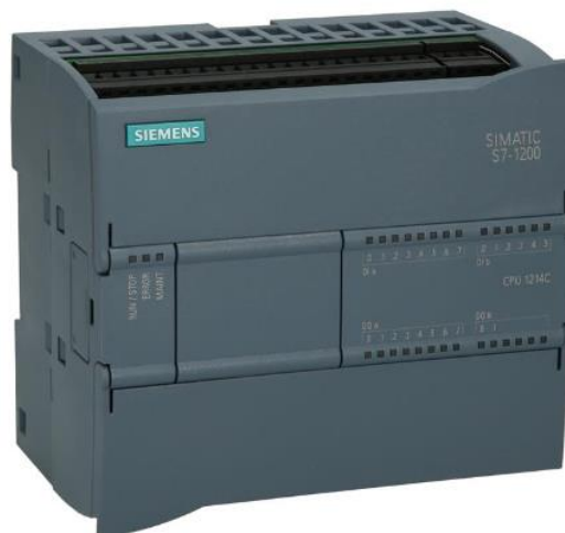
Figure 3.8 : Automate SIMATIC S7-1200 [12]
