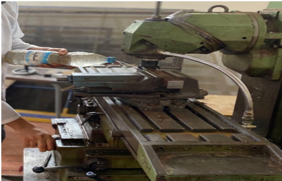
Figure 5. 5 Surfaçage et lubrification manuelle
