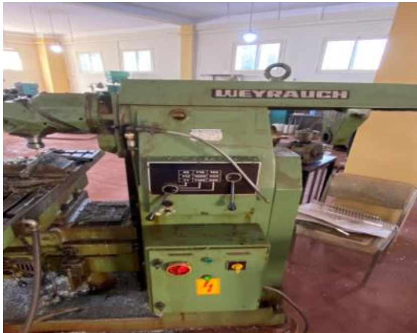
Figure 1. 5 Fraiseuse universelle WEYRAUCH FR-U-1100
