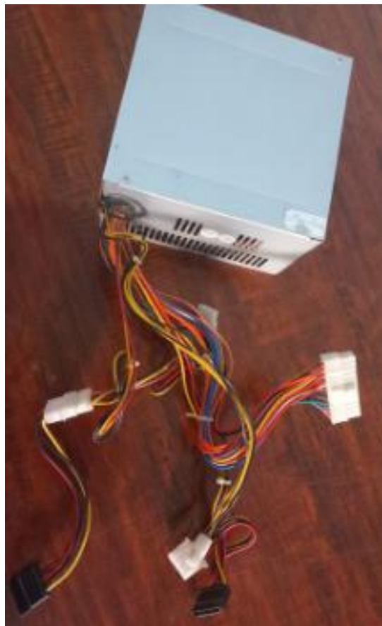
Figure IV-1 : ATX power supply
