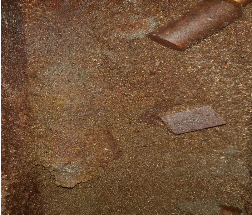
Figure V.3 Accumulation des copeaux
