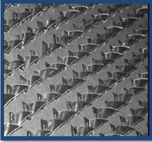
Fig.II.1. Disposition des obstacles DCL. [29]
