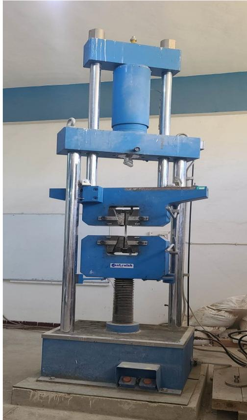
**Figure IV-23 : Machine traction 600kg/N**
