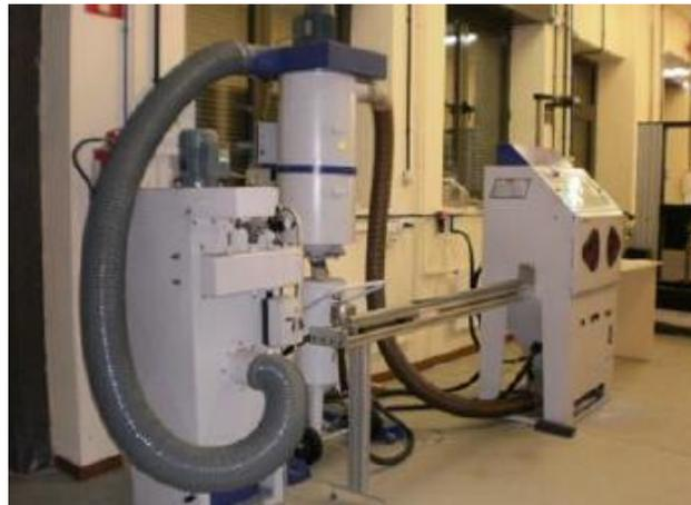
Fig.2. 2 Machine de grenailage
