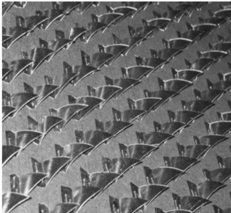
Figure II.2 : Disposition des obstacles DCL
