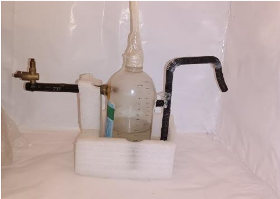
Figure III-6 : water bottle method for the Biogas measurement
