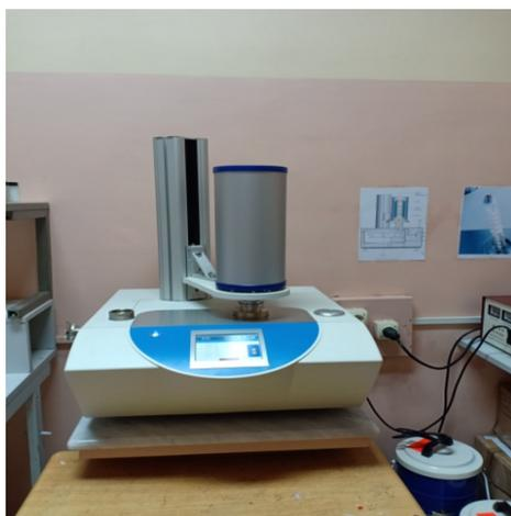
**Figure 8.** Appareil ATG type LINSEIS.STA.PT.1600
