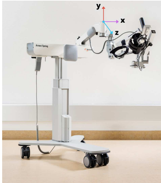
Fig. 1.1.: Armeo Spring device, a passive orthotic exoskeleton for upper limb rehabilitation training. The reference frame attached to the shoulder sensor defines all the positional measurements recorded in the dataset used for this study. Image courtesy of Hocoma Inc. Switzerland.
