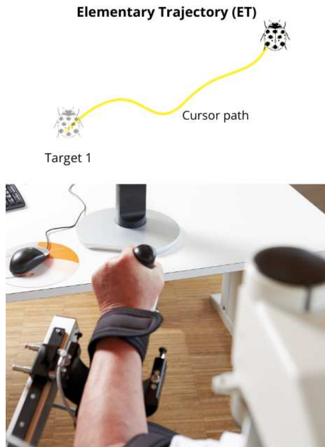
Fig. 1.3.: The pointing task generates the data. Patients are using the exoskeleton to drive the cursor and point out targets. The trajectories of the end effector during these sequences of movements constitute the elementary study units noted ET. The Armeo Spring picture is courtesy of Hocoma Inc. Switzerland.
