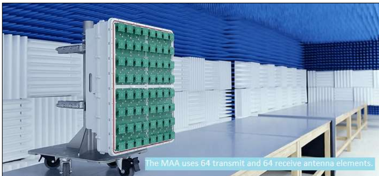
Figure II.3 : Antenne massive MIMO de Nokia [16]
